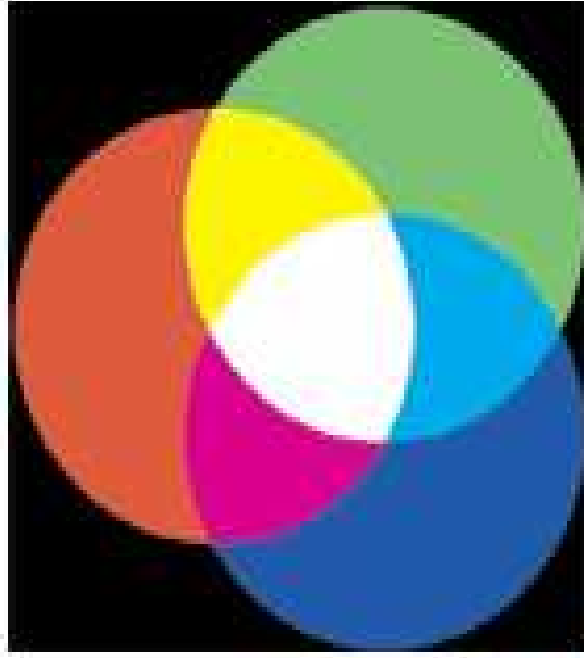
Figure 4-5: The RGB color model is based on red, green, and blue light.
