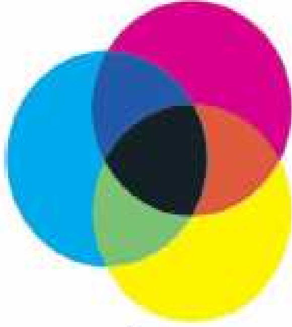
Figure 4-6: The print color model is based on cyan, magenta, and yellow ink.
